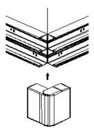
Positioning of the trunking to the wall before clipsage of the external angle
