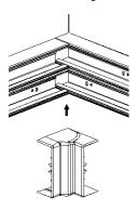
Positioning of the trunking to the wall before clipsage of the internal angle
