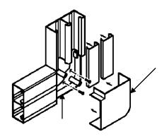
Positioning of the trunking to the wall before clipsage of the flat angle
