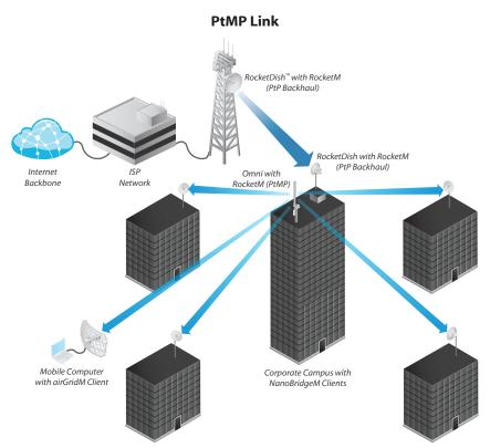
The combination of the airMAX Omni Antenna with a Radio radio provides 360° coverage and utilizes airMAX technology to provide carrier-class performance and power.
