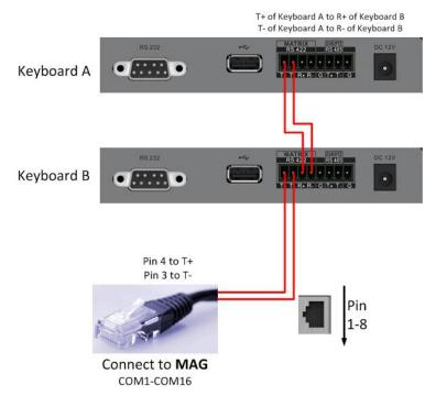
Figure 3-7 Connection between Cascaded Keyboards and MAG
